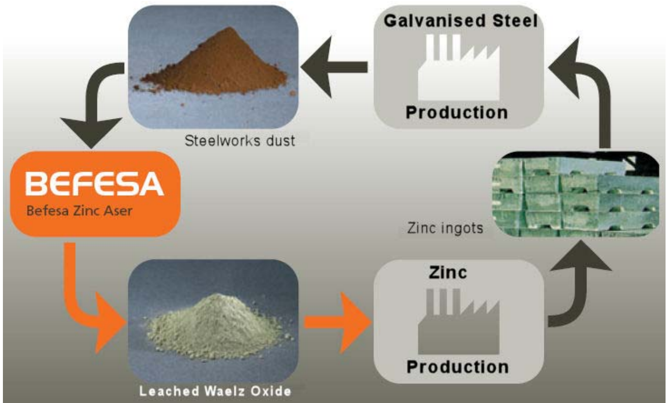
Galvanised steel zinc recycling circuit
